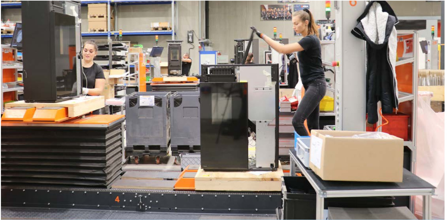
An assembly line contains six modules each with two lift tables. They move 2 cm up over the chain conveyor at the station. Then the employee can lift, turn and swivel the table, attach mechanical parts or electronics. At the end the table is put into the locked position. At the touch of a button it moves down again onto the chain and is transported to the next station.
