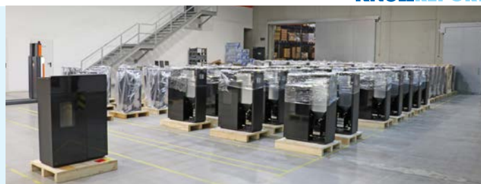
The main bodies required in the morning are made available in the buffer zone. The fully assembled stoves are also stored there temporarily.
