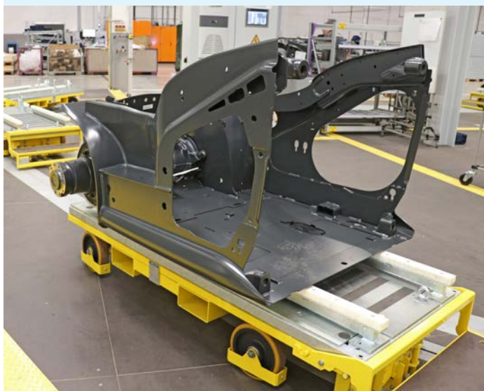
For the TS-Z mounting trolley, KNOLL developed a quattro steering that enables driving on curves.
