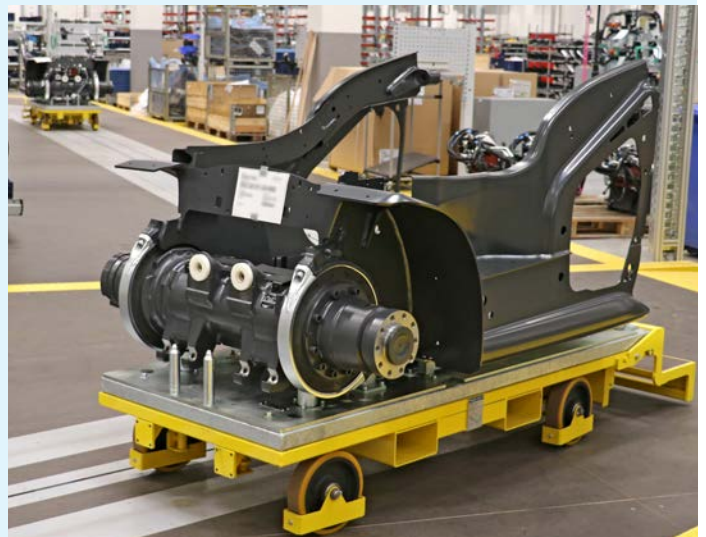
The frame components are assembled at eight stations. Each one is five meters long and takes nine minutes to traverse.
