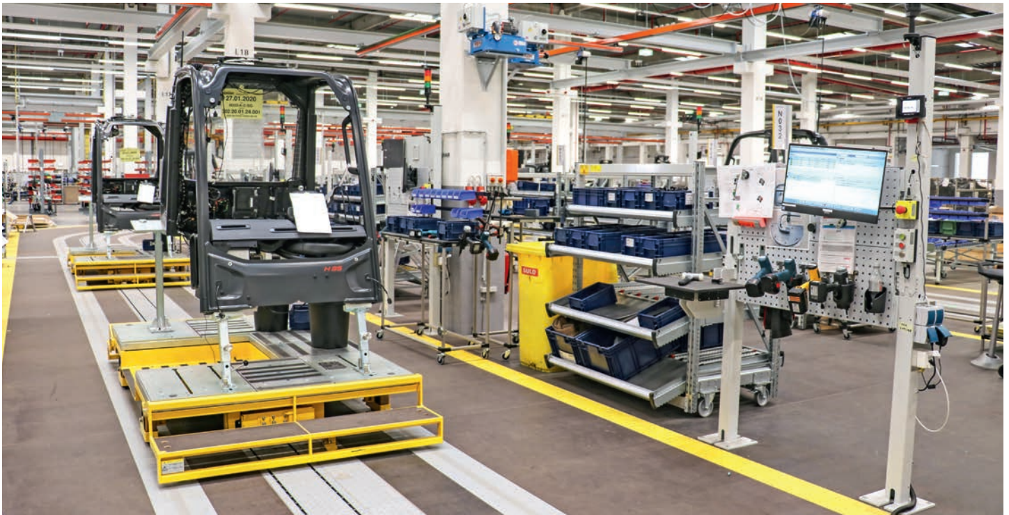
For a new lift truck generation that is built by Linde in the Aschaffenburg "Plant 2," KNOLL developed two pre-assembly lines – for the frame and the overhead guard (in the picture).
