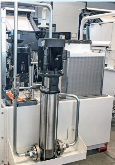
Modular construction: a console with high-pressure pump can be retrofitted at any time.
